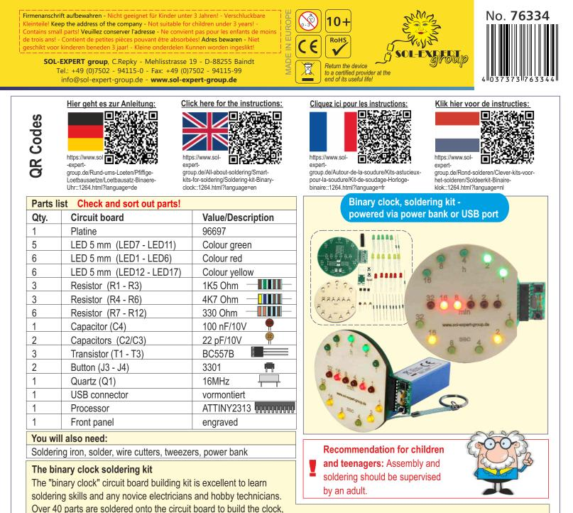
including a preprogrammed microprocessor. This enables showing the "binary" time through LEDs. One LED row is assigned to the hour/minute and one to the seconds. The actual time is set with buttons. The "binary clock" electronics building kit is powered via power bank or via USB port. This eliminates costly batteries. The included plywood front panel shows the binary values. These can then be converted to decimal values. Dimensions: 100 x 80 mm.
